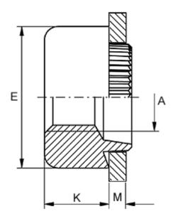
Female thread A = M3,5Height K = 4.0Outer diameter E = 10.0Plate thickness = 4.1 to 4.3
